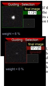
If the cursor is set to the star number and **SET** is pressed, the image of the respective star is displayed (here star 1 from 21), and the weight for its contribution to the multistar. The smaller window shows its position on the sensor.
