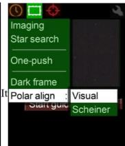
The respective screen is grouped with the Scheiner method in: Imaging menu, Polar alignment submenu. Place cursor on Polar align and press **SET** to unfold the submenu. Press SET again to enter.
