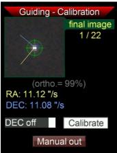
Set the cursor on **Calibrate** and start calibration by pressing **SET**. The sequence takes a few seconds and ends displaying some results. First, the orthogonality of the DEC and RA movements, and the respective speed the multistar movements in each axis.
