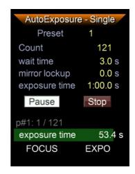
You can pause and restart the exposure sequence at any time. Two signals are sent to the DSLR: First, the focus signal (like half pressing the exposure button) and ESC lights up, then the shutter release signal and SET also lights up. If you want to use mirror lock, you need to activate it in the DSLR. The value 0.0s means no mirror lock. We do not recommend mirror lock with long exposure times. Mirror shake is more of a problem with very short exposures.
