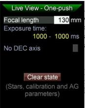
At the **onepush** screen, to the right of Start guiding, there is a little box containing three dots. Set the cursor onto it and press **SET** to enter a submenu, which allows to quickly enter some basic values if needed. It's a **shortcut**, we will discuss and set these values now at the menus that are their homescreens.
