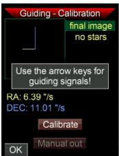
At the bottom of the page there is the **Manual out** button. This is an important tool to check the connection to the mount. Set the cursor and press SET, a box appears telling you to now transmit the ST4 signals by pressing the directional buttons. Check if the multistar moves when you output the signals manually. Exit this mode by pressing **ESC** (OK).
