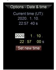
Mgen3 has a real-time clock built in, that is powered by an internal battery and continues even after shutting down. The battery is CR2032 type and can be found on the backside of the board. You need to remove the board to change it, if necessary.
