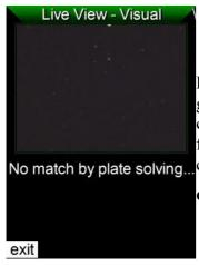
**Remark:** While moving the guidescope, the exposures are constantly going on and the stars will be smeared. This screen tells you that the current frame could not be platesolved. Just wait a second to get the next frame to be measured. Also, if the guidescope is not pointed at the area covered by star data, this message will be shown.
