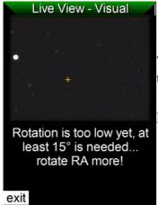
The location of the pole is now saved and the mount's RA axis' point on the sky should be determined. To do this you should turn RA for at least 15 degress. Make sure not to touch DEC.
