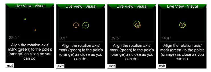
When getting the RA axis near the pole, the view zooms in automatically and circles appear around the two crosses. The better the match, the smaller the adjustments must be done to home in. A precision smaller than 5arcmin is aptly sufficient for astrophotography when using an autoguider, but you may try how close you can get. Press **exit** to quit.
