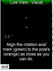
The live view disappears and the two points can be seen, auto zoomed. The distance between them is displayed too, so that you know if adjusting the mount's Alt/Az in a direction is good or you need to adjust it in the opposite direction. Start adjusting Alt/Az screws on your mount now and watch the points approaching each other and the number getting smaller. The goal is to get the green cross (RA axis) to match the orange one (the pole).
