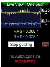
The live picture is then replaced by the guide graph, and at the bottom, Autoguiding is displayed in red blinking letters. You may now start the exposure sequence with your camera, and the status is shown here, too.
