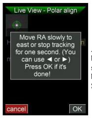
• press **calibrate**. The Mgen-3 needs to know how the pixel rows of its camera are related to the mounts axes. This is done by a small calibration routine. You only need to do it once at the beginning of every polar alignment session.
