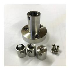
Slip the spacer Inlay over the worm and align the holes with the threads in the coupler, so the screws are able to contact the worm directrly. Using the proper length hex screws (2 pcs, 180° positions) fix the coupler to the worm, but at first not tightly. Move the focuser worm manually to let the coupler align with the worm, when done only then fix the coupler to the worm tightly, and the motor to the worm housing.
