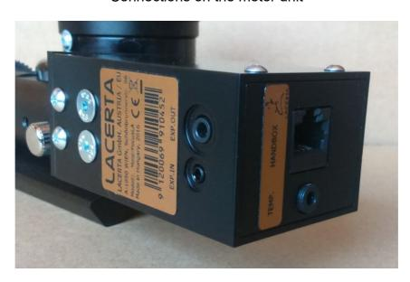
left side: 2,5mm stereo socket (from MGEN's camera port)
