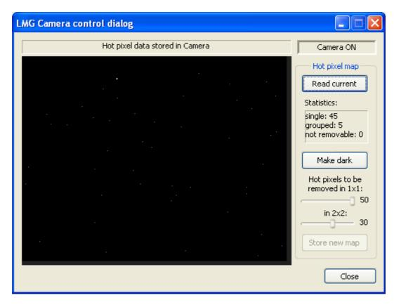
"Statistics" gives some info about the amount of different hot pixel types. Single hot pixels are surrounded with normal (non-hot) pixels. A grouped hot pixel is such that it has at least one neighbouring hot pixel. These could be cosmetized as well but with less efficiency, since there are less surrounding good pixel information. Not removable hot pixels are totally surrounded by another hots, these are very rare and won't be cosmetized at taking frames.
