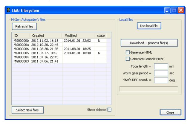
On the left side the file list is shown that are stored currently in the autoguider. If HC is not connected to PC or turned on, the list is empty and buttons in the group box don't have any effect. The PC application can't access the files in the autoguider (seen as there were no files in it) if:
