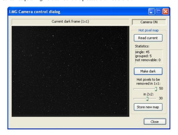
The displayed image is reduced in size by a factor of two, so each pixel shows the maximum of a 2×2 pixel block of the CCD. That's why You can see a lot of gray ("warm") pixels besides the hots. Maximum must be shown to see every single hot pixel left (not cosmetized yet).
