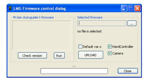
On the left box information or error is displayed about the autoguider's current firmware. On the right, You can select a local firmware file (on Your PC) and get it uploaded into the autoguider.
