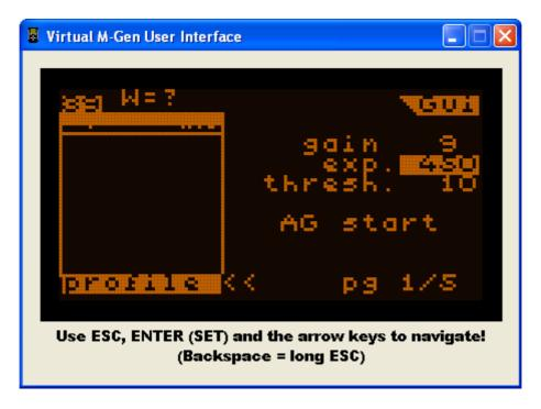
The display here is exactly the same as on the HC's LCD display. The buttons are replaced by the PC's keyboard with the following mapping:
