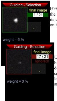
If the cursor is set to the star number and **SET** is pressed, the image of the respective star is displayed (here star 1 from 21), and the weight for its contribution to the multistar. The smaller window shows its position on the sensor.
