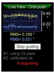
The live image is replaced by the guide graph, showing the progress of the autoguiding and displaying the rms deviations. You may also stop and resume guiding from here. If a new starfield is detected, a new star search and calibration takes place automatically. If detection fails, you may go to the Star search page and start the Star search there manually. Normally, the whole one-push sequence from start to autoguiding takes only about 30 seconds, no more.
