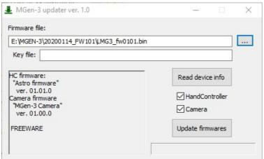
Start the Updater.exe, the interface pops up and to the right you find a small box with 3 dots. Click on it to select the firmware.bin file and confirm. A second box pops up, here load the keyfile. Check if **HandController** and **Camera** are both ticked, and choose **Update firmwares**.
