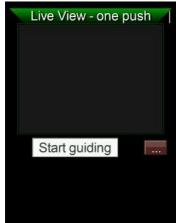
A short press of the **ESC** button turns on the Mgen-3, and after the splash screen the **One push** screen is displayed. What you see here is a live picture from the camera, containing stars. Its a black and white picture because the Mgen-3 camera has a very sensitive monochrome sensor.
