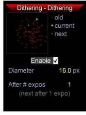
In the box in the upper left there is a graphic display: The previous positions are represented by little red crosses, the actual position by a yellow one, and the next calculated position by a green one. As dithering progresses, a little cloud of red crosses is built up showing the distribution of the points.
