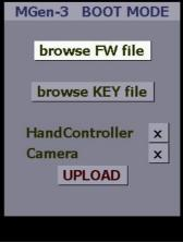
Alternatively: if you do not use Windows, you may download the firmware and keyfile, and copy it to the microSD card – to the basic (root) directory. Make sure the keyfile really has the .mg3key file extension and nothing else (careful with MacOS!). Insert the microSD card and enter Boot mode. Go down to device info and press the RIGHT key. On the new screen choose Upload new and browse the files on the subscreen. Tick HandController and Camera. Press UPLOAD to update the firmware.
