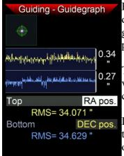
By default you see the positions of the multistar displayed, showing the deviations from the zero line. RA is the upper, DEC the lower graph. The graph is updated every guide cycle and shows about the last 220 positions.
