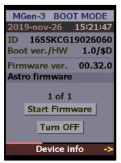
Its most easy to update your Mgen3 using a Windows PC. You need to install the FTDI driver to communicate with Mgen (see page 3). Connect your Mgen3 inclusive camera and connect via USB. Enter Boot mode to get it ready for receiving the data. Place the downloaded firmware and freshly downloaded keyfile in the same folder as the updater App (that is usually contained in the firmware zip file, or download it from the support site, too).
