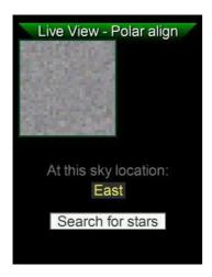
A new screen appears. Now turn the mount to the Eastern or Western point most near horizon in your reach. Keep on the equator, so do not move DEC. Select your location on this screen and press **Search for Stars**.
