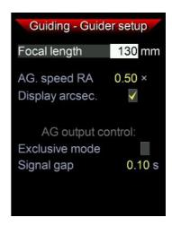
Check if the default values fit or need to be corrected for your setup. A 50mm finder usually has a focal length of 180mm, and a 30mm finder is usually 120mm. A Synta 50mm ED finder has 240mm. The autoguiding speed is usually 0.50x sidereal rate.
