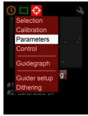
The guiding parameters are values basic to guiding. Measured deviations of the multistar must be converted into correction signals, and how the Mgen-3 does that can be adjusted here. The default values are configured to work well in most situations, but with the Mgen-3 it is also possible to fully control the algorithm manually. The values chosen here apply also in one-push autoguiding.
