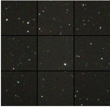
Now focus in the **center** of the image. If the stars are well rounded in the corners, you have hit the working distance well. If they appear flattened towards the center, as in this example, the corrector has too strong an effect and the distance must be reduced. If they are elongated towards the center, then the corrector has too little effect and the distance must be increased.
