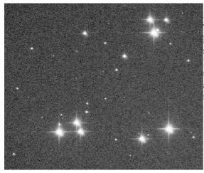
To prevent dew condensation, it is practical to attach a heater to the secondary. However, if the heater is too strong, the warm air rises into the optical path and causes light bursts on brighter stars in the entire image. If you tilt the tube, the direction can change because the warm air always rises. So it is important to heat only as much as necessary.
