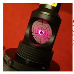
The tilt of the primary is now adjusted so that the laser beam returns to the laser itself, exactly in the hole where it originates. This ensures that the secondary is centered in front of the focuser and correctly aligned with the primary, and that the optical axis of the primary is correctly guided into the axis of the focuser.
