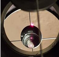
View from above into the Newtonian tube. You can see the primary with the center marking, where the laser beam does not yet hit the very center.
