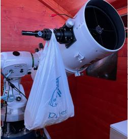
spider vanes well tensioned and secondary base tightened? primary without lateral play in the cell?
