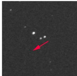
For **visual observation** at high magnification, it is sufficient to adjust the remaining coma directly using an observed star. Just adjust the primary so, that the star moves in the same direction as the coma tail (red arrow).
