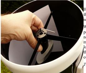
Hold and align the secondary base with one hand and adjust the center screw with the other until the laser beam hits the secondary at its mark.
