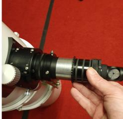
With the OctoPlus focuser, the extension tube first takes over the guidance, the corrector fits and can only tilt by the slip dimension. The clamping alone is not precise enough for the alignment. Only such a slip fit or a screw connection is sufficiently reproducible. Here in the picture, the laser is screwed to the first GPU prototype and is inserted into the focuser.
