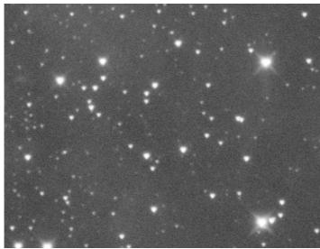
**Strained optics**: If the retaining clips of the primary are tightened too much, the mirror will deform. They must not touch the primary at all, only secure it against falling out. A deformed optics produces deformed stars in the whole image.
