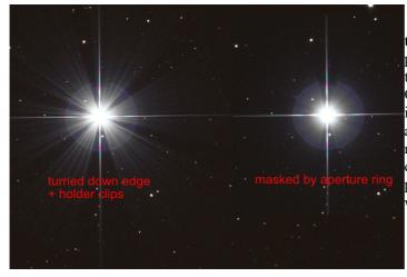
turned down edge: After the grinding process, some mirrors have a small zone on the edge that has been ground too flat. Often it is only half a millimeter. The light is transported far out of the diffraction disk and floods the surrounding image field. The retaining clips cover this in their area and dark recesses form. Masking with black pencil or a diaphragm eliminates the effect without costing much aperture.
