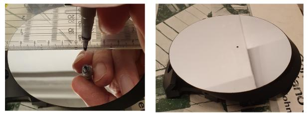
Most secondaries have already been glued to their mounting base with this offset by the telescope manufacturer, so you simply attach the base to the spider and the spider legs can stay nice and straight. So setting the correct position of the secondary in front of the focuser is now easy, the laser just has to hit this point. But it also has to hit the primary center. So there is only one position of the secondary where this really happens. This position has to be found.
