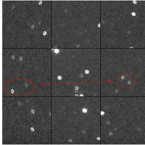
Now we look at the **edge of the field** with the 4 image corners and **compare the shapes** of the star disks. In the image corners, a certain residual astigmatism is normal, namely **intrafocally** the star discs are flattened towards the image center.
