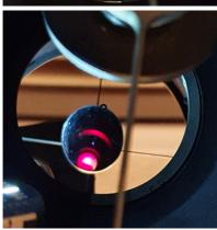
Suitable illumination of the secondary surface should be provided, whereby the primary can be used as a reflector.
