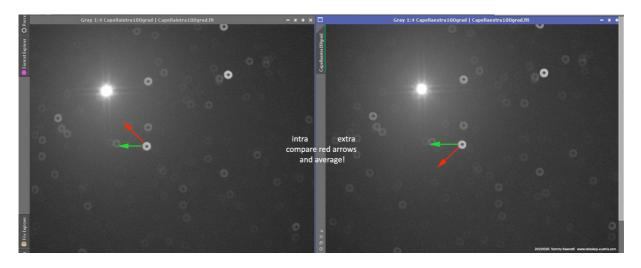
For more details see the hints below! This more accurate method does not have to be used if the coma is obvious from the uneven brightness distribution of the star disks. It is usually sufficient to use it at the end of the adjustment.
