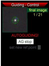
When autoguiding is started, AUTOGUIDING! appears and blinks, and a red cross marks the set point where the star should be kept.
