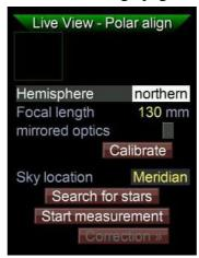
Polar aligning a mount usually is done before autoguiding, so after startup you can switch directly to this page. The screen looks loaded at first, but all entries are in a logical sequence and allow to do the adjustments in just a few steps:
