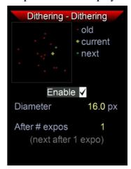
If enabled, the MGEN-3 will shift the guide star automatically a little bit after the specified number of exposures. You can observe the shifting on the active LEDs of the directional buttons when the ST4 output is activated immediately after the DSLR exposure has ended.
