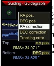
If the cursor is on **RA pos**., you may press **SET** and a box pops up. Here you can choose what kind of graph should be displayed – correction means the length of the respective AG signals, and tracking error are the summarized corrections.
