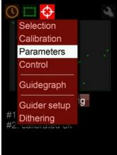
The guiding parameters are values basic to guiding. Measured deviations of the multistar must be converted into correction signals, and how the MGEN-3 does that can be adjusted here. The default values are configured to work well in most situations, but with the MGEN-3 it is also possible to fully control the algorithm manually. The values chosen here apply also in one-push autoguiding.
