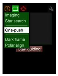
Here you can shift the cursor by pressing the directional buttons  $UP \triangle$  and  $DOWN \lor$ . By LEFT  $\triangleleft$  and RIGHT  $\triangleright$  you can change to other main menus.
