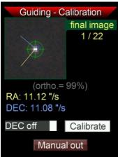
Set the cursor on Calibrate and start calibration by pressing SET. The sequence takes a few seconds and ends displaying some results. First, the orthogonality of the DEC and RA movements, and the respective speed the multistar movements in each axis.
