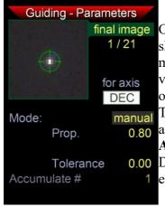
On the DEC page the standard mode is currently **manual** only. The DEC shows neither periodic error nor overtones, but static drifts or erratic movements. So an integral term does not make much sense. Instead, a value of 0.8 for proportional will suit most situations. In the case of overreaction you may lower this value to avoid oscillation of the mount. The tolerance can be left at 0.00, or increased if corrections in the DEC axis need to be dampened. For advanced users only!
