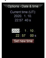
Mgen3 has a real-time clock built in, that is powered by an internal battery and continues even after shutting down. The battery is CR2032 type and can be found on the backside of the board. You need to remove the board to change it, if necessary.
