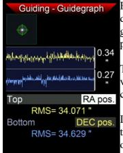
By default you see the positions of the multistar displayed, showing the deviations from the zero line. RA is the upper, DEC the lower graph. The graph is updated every guide cycle and shows about the last 220 positions.
