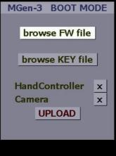
Alternatively: if you do not use Windows, you may download the firmware and keyfile, and copy it to the microSD card – to the basic (root) directory. Insert the microSD card and enter Boot mode. Go down to device info and press the RIGHT key. On the new screen choose Upload new and browse the files on the subscreen. Tick HandController and Camera. Press UPLOAD to update the firmware.
