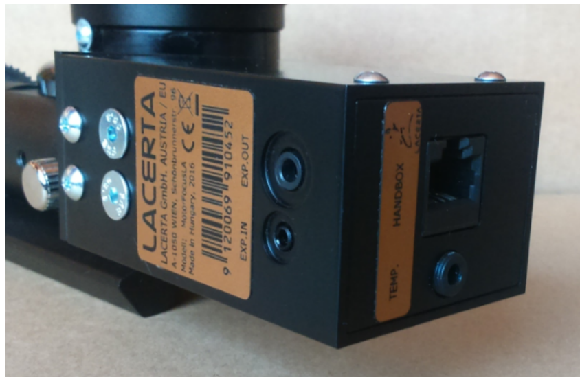
Anschlüsse am Motor
